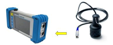
Procedure Insert the plug of the PAM CORR-2 cable into the microphone connecting socket 4 on the HLE 7000. Observe the marking. You must feel the plug engage.
