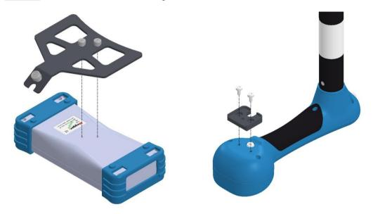
In the next step, the operating unit can be screwed to the underside of the carrying pole.
