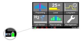
As soon as the battery of the device has reached a minimum, a message appears on the screen. The device should then be charged as soon as possible.
