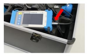
Charging on the mains The device can also be connected to the mains for charging. Use the supplied power adapter and the VK 130 connection cable.
