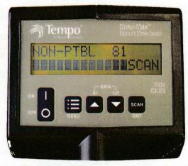
**Scan Mode:** Automatically determines marker type detected (power, water, sanitary, telephone, gas, CATV, non-potable)
